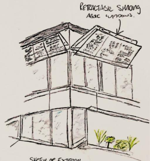
SKETCH OF EXTERNAL SHADING ON WINDOWS, MATCHES CORRESPONDING SECTION
